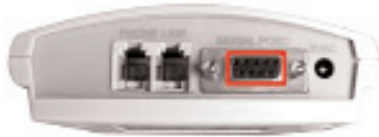
Connect to Serial Port on the modem
