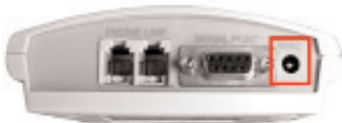
Connect power cable to the Power socket on the modem
